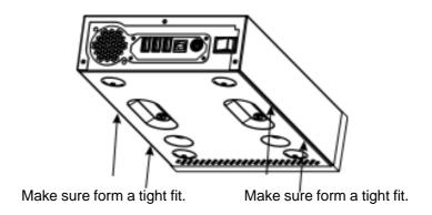
d) Replace the three screws which were removed in Step 1 from the back of the enclosure.
